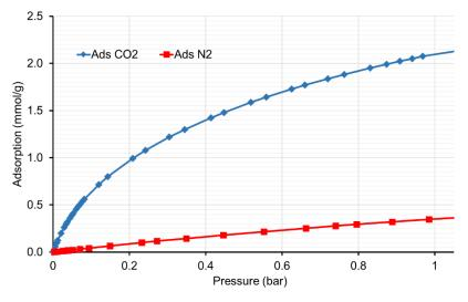
Industrial performance of Starbon® A800 adsorbing CO2 at 25 °C
